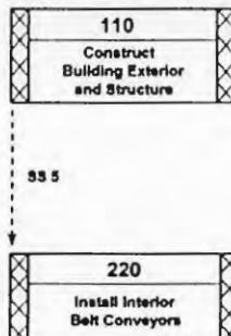
*Install Interior Belt Conveyors can start five days or more after Construct Building Exterior and Structure starts.*
